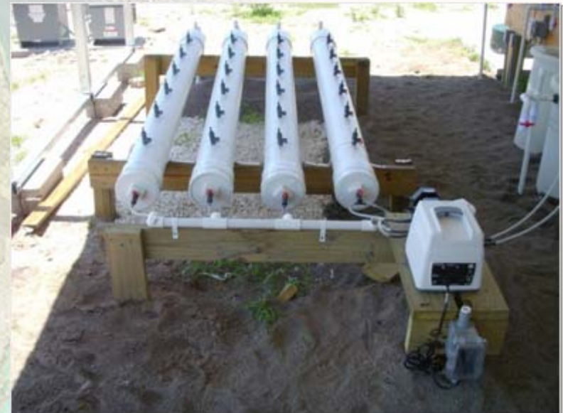
Stage 2 Saturated Biofilters
