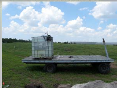
250 gallon tank with bromide solution
