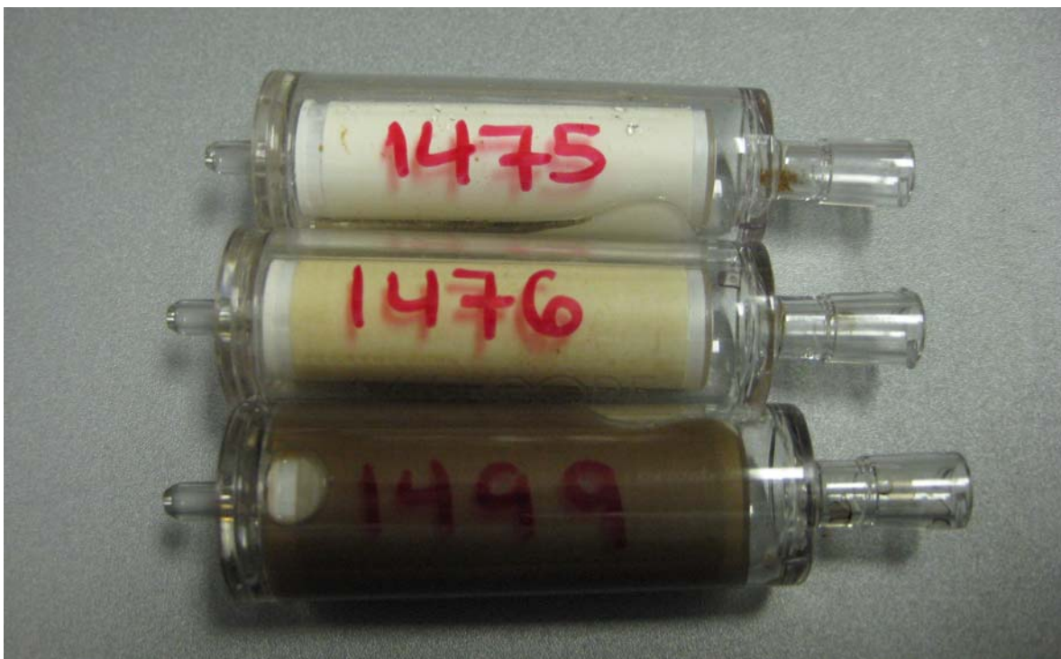
Figure 8. Filters capsules used to prefilter OSTDS samples for CDOM absorption determination illustrating the range in particulate color.
